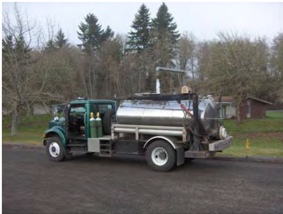
a 1,500 gallon tanker truck with a screened top entrance for ventilation and loading fish, an oxygen system, and
