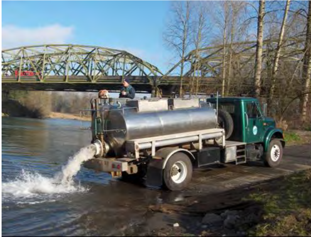
a rear gate designed to offload fish to locations designated by the Washington Department of Fish and Wildlife.
