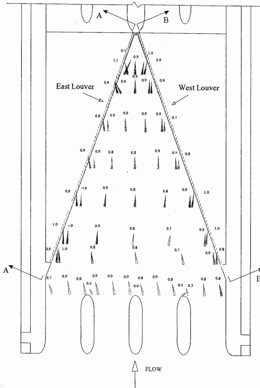
Figure B-1: X-Y Vector Velocity (m/s) at Elev. 395.6 ft (Q = 1290 cfs)
