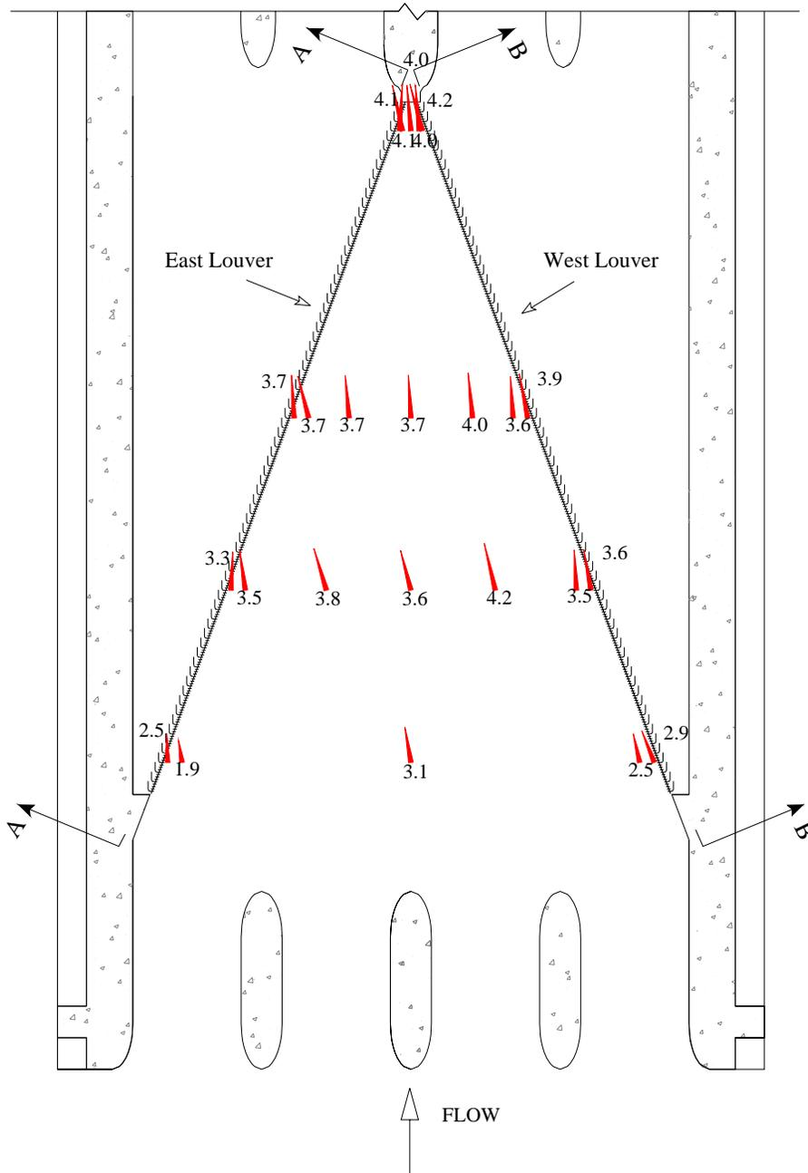
**Figure 3** – Field measured velocity at elevation 416.4 ft (msl) and 5,835 cfs. Velocity magnitude shown in feet per second.
