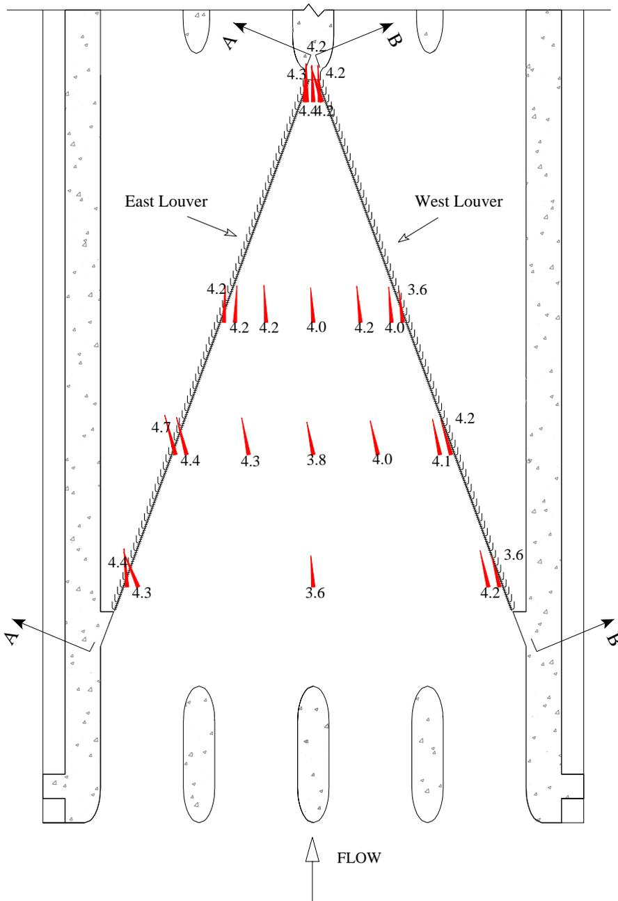
**Figure 2** – Field measured velocity at elevation 402.3 ft (msl) and 5,835 cfs. Velocity magnitude shown in feet per second.
