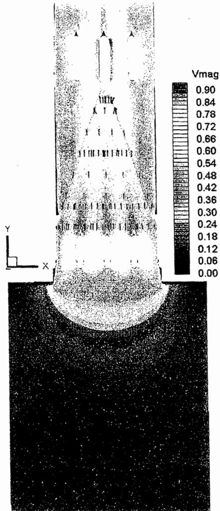
Figure C-10: Verification Run02 (Q=2580 cfs, elev. 395.6 ft, Vmag in m/s)
