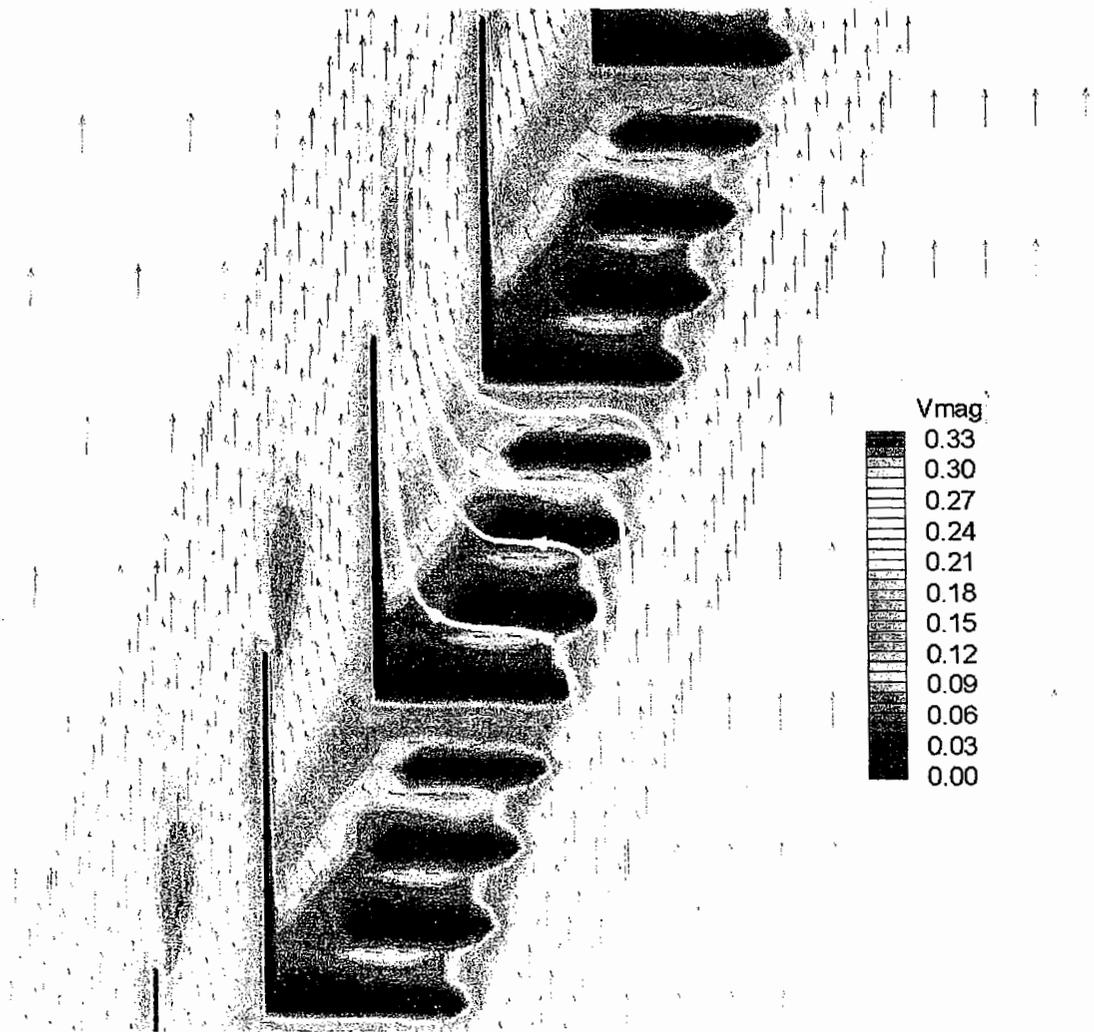
**Figure C-20: Run05 louver zoom (Q=1290 cfs, elev. 402.7 ft, no-slip louvers, Vmag in m/s)**
