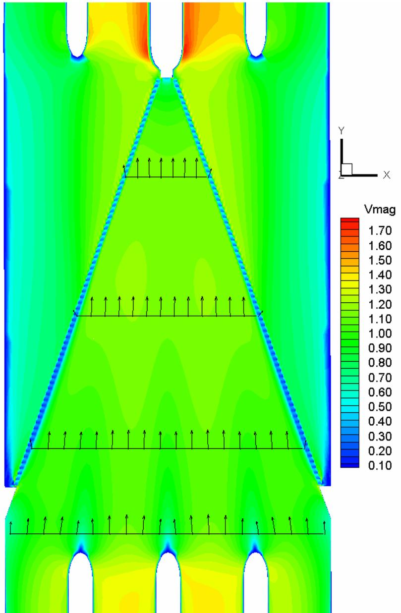
**Figure 8** – CFD predicted velocities at elevation 402.3 ft (msl) and 5,000 cfs.
