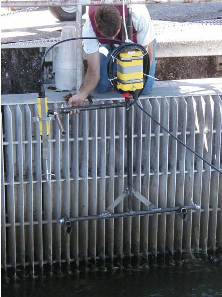
**Photo 1** - ADV probe mount designed to deploy ADV by indexing on louver vanes.
