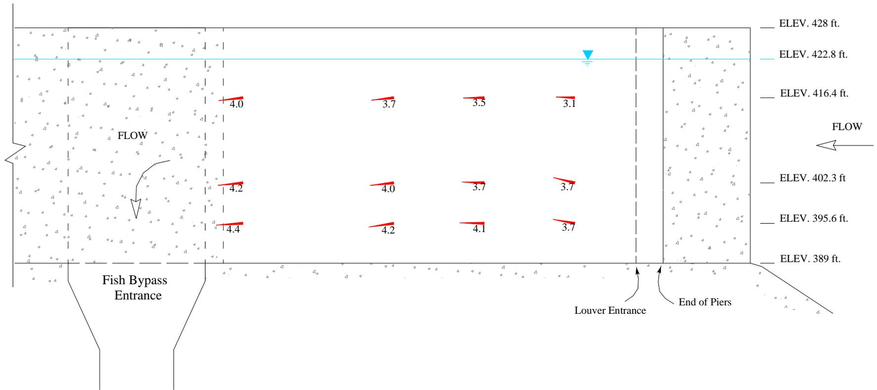
**Figure 5** – Field measured velocity along longitudinal centerline of intake bay at 5,835 cfs. Velocity magnitude shown in feet per second.
