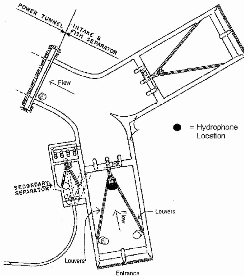
Figure 13: Plan view of the Mayfield louver array and hydrophone locations.
