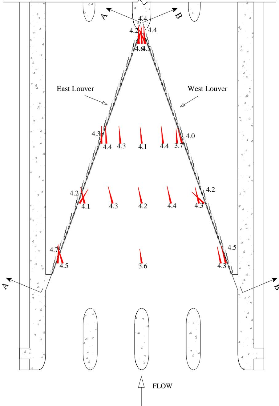
**Figure 1** – Field measured velocity at elevation 395.6 ft (msl) and 5,835 cfs. Velocity magnitude shown in feet per second.
