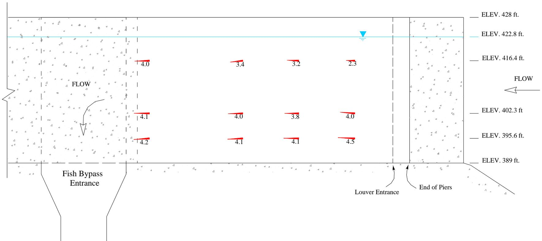
**Figure 4** – Field measured velocity along east wall at 5,835 cfs. Velocity magnitude shown in feet per second.
