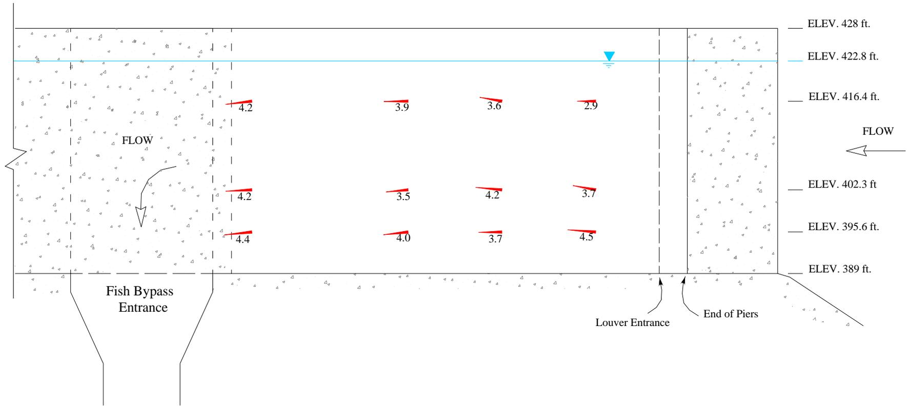
**Figure 6** – Field measured velocity along west wall at 5,835 cfs. Velocity magnitude shown in feet per second.
