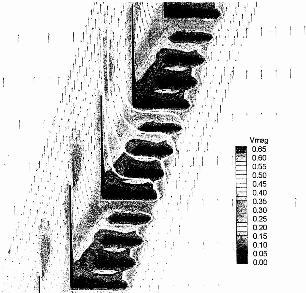
**Figure C-22: Run06 louver zoom (Q=2580 cfs, elev. 395.6 ft, no-slip louvers, Vmag in m/s)**
