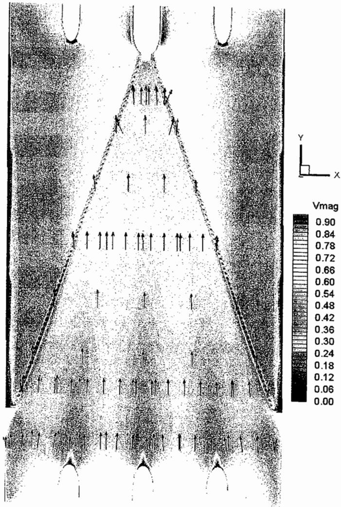
Figure C-11: Verification Run02 zoom view (Q=2580 cfs, elev. 395.6, Vmag in m/s)
