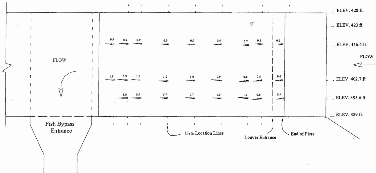
**Figure B-9: X-Z Vector Velocity (m/s) at West Louver (Q = 1290 cfs)**
