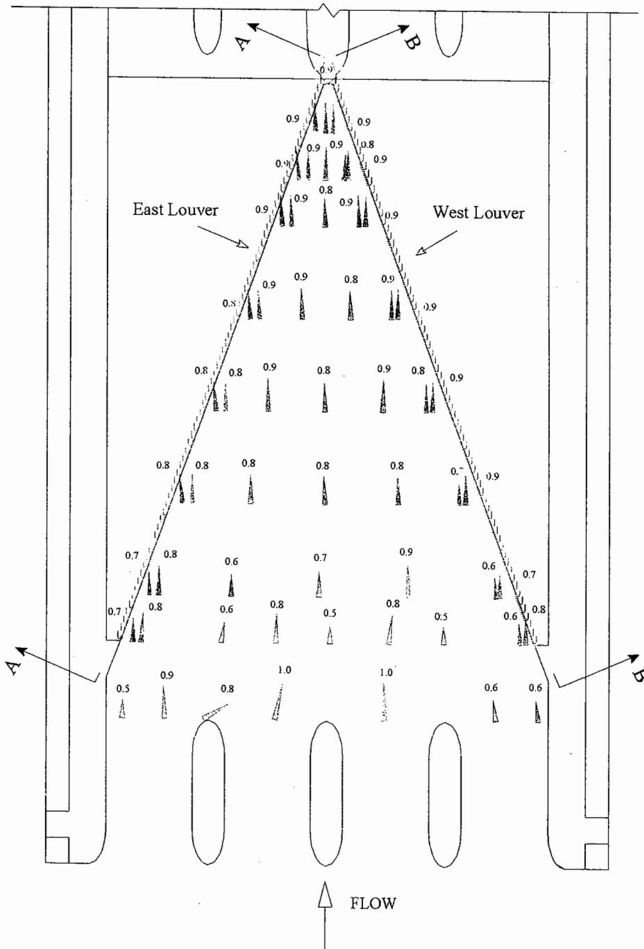
Figure B-3: X-Y Vector Velocity (m/s) at Elev. 416.4 ft (Q = 1290 cfs)
