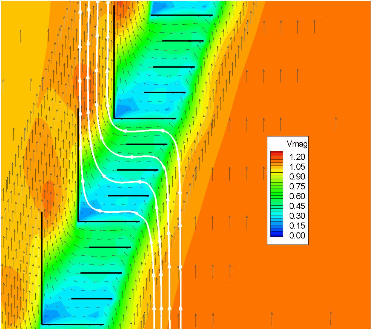
**Figure 12** – CFD measured velocities through louver vanes at elevation 416.4 ft (msl) and 5,000 cfs. Velocity magnitude shown in meters per second.
