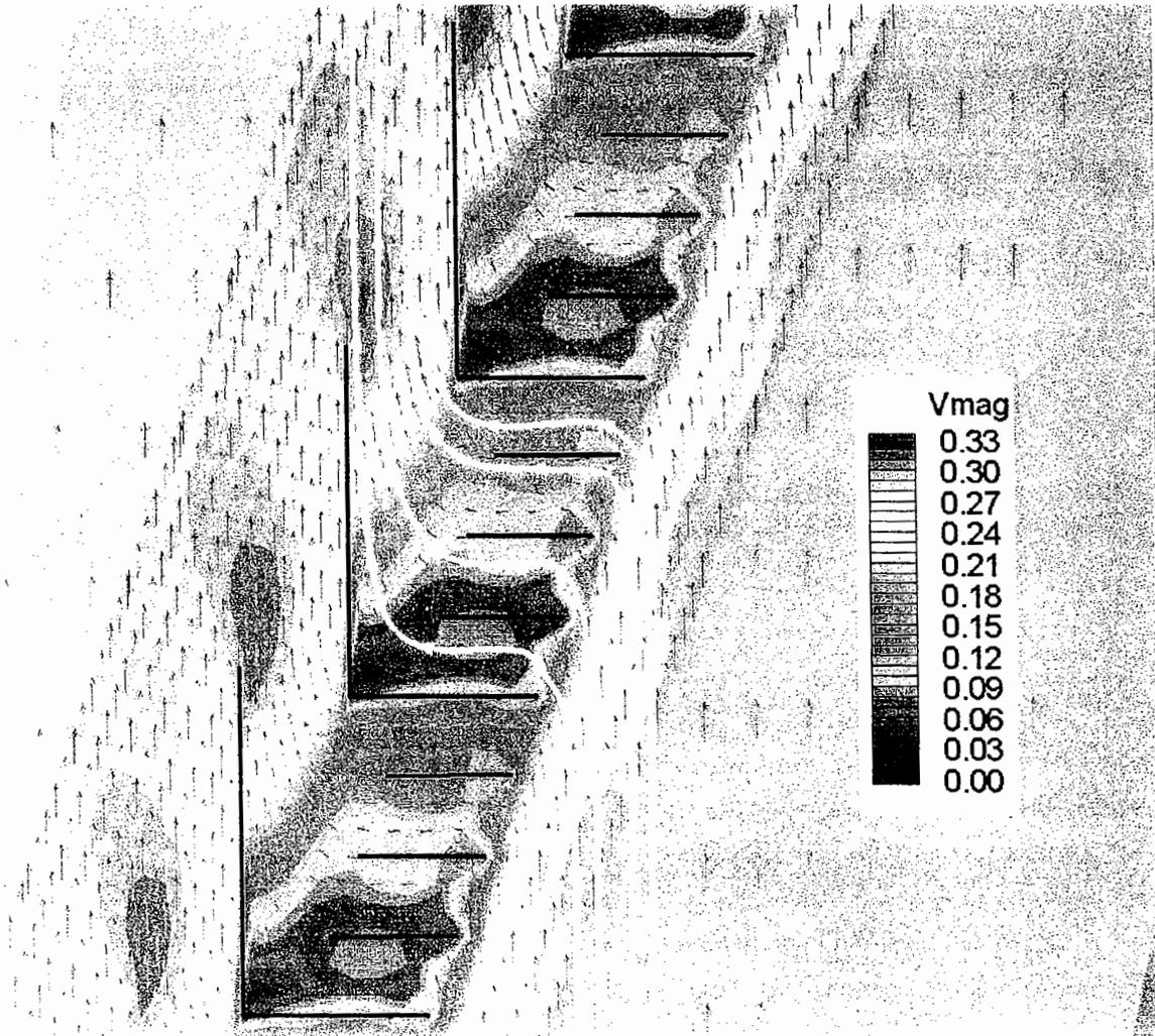
Figure C-6: Verification Run01 louver zoom (Q=1290 cfs, elev. 402.7 ft, free-slip louvers, Vmag in m/s)
