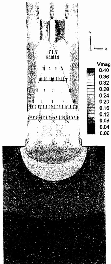
Figure C-1: Verification Run01 (Q=1290 cfs, elev. 395.6 ft, Vmag in m/s)
