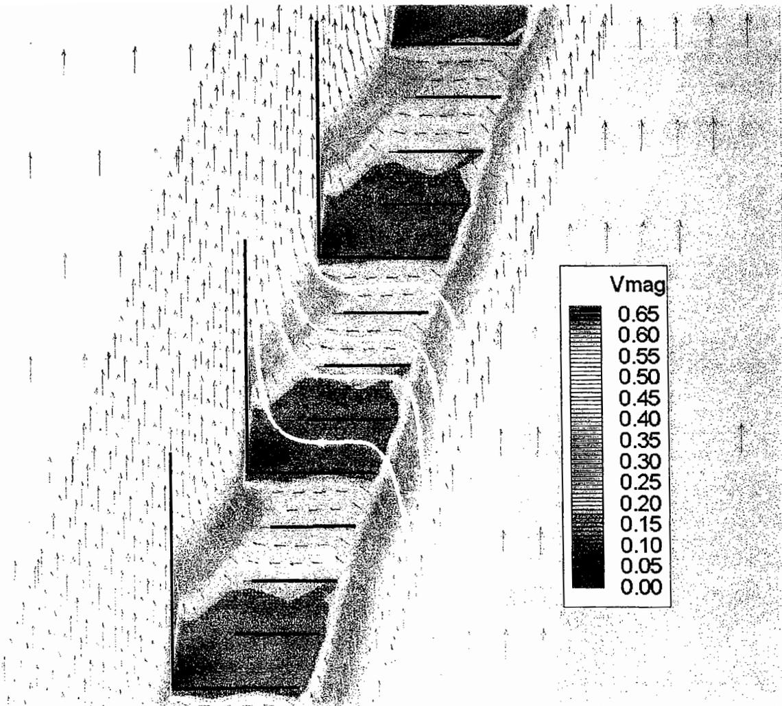
**Figure C-18: Verification Run02 louver zoom ( $Q=2580$  cfs, elev. 416.4 ft, free-slip louvers, Vmag in m/s)**
