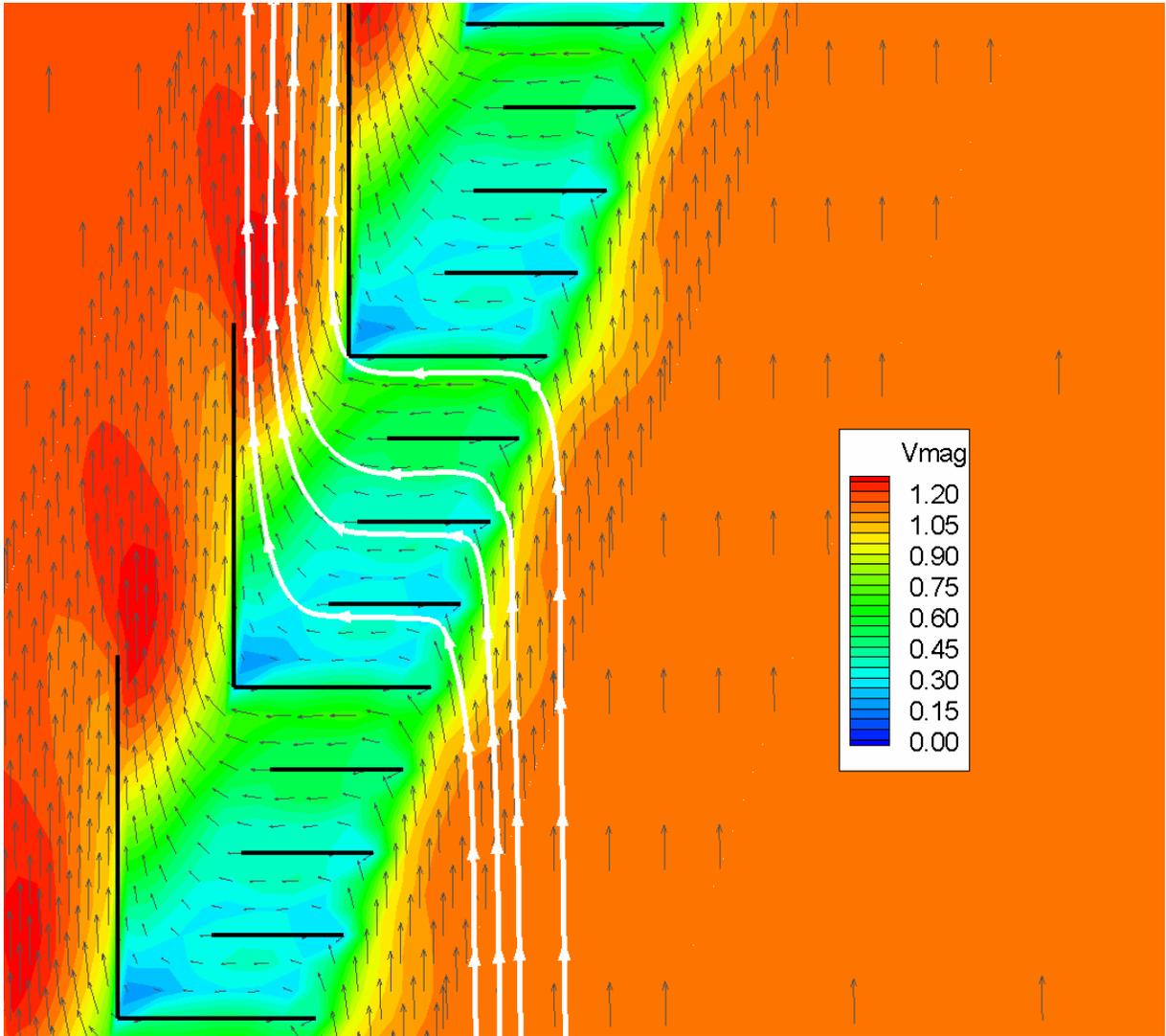
**Figure 10** – CFD measured velocities through louver vanes at elevation 395.6 ft (msl) and 5,000 cfs. Velocity magnitude shown in meters per second.
