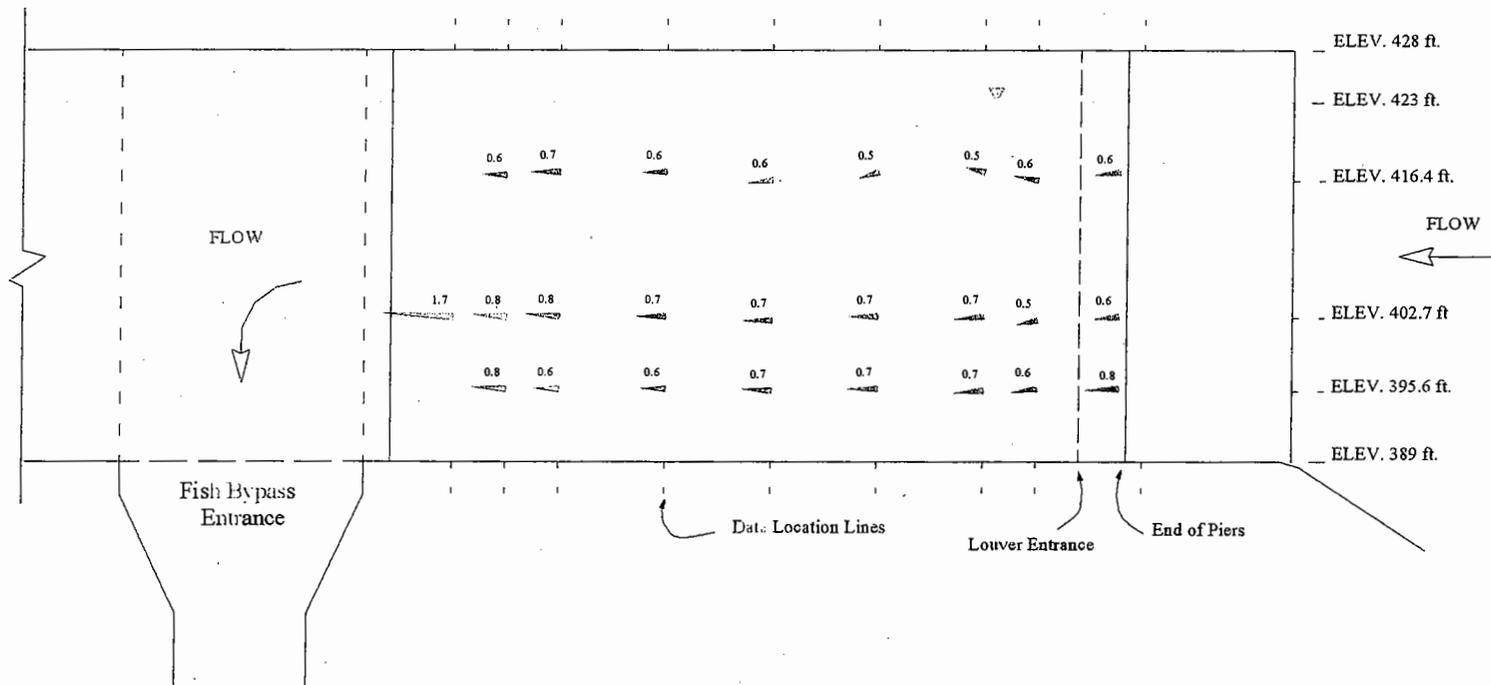
**Figure B-7: X-Z Vector Velocity (m/s) at East Louver (Q = 1290 cfs)**
