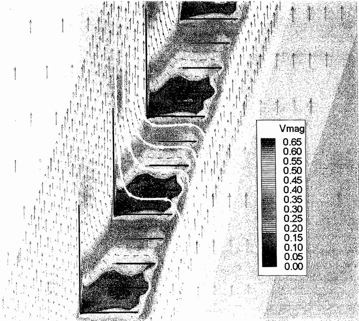
**Figure C-15: Verification Run02 louver zoom (Q=2580 cfs, elev. 402.7 ft, free-slip louvers, Vmag in m/s)**
