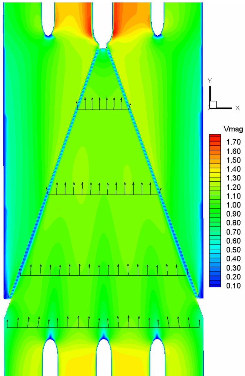
**Figure 7** – CFD predicted velocities at elevation 395.6 ft (msl) and 5,000 cfs. Velocity magnitude shown in meters per second.
