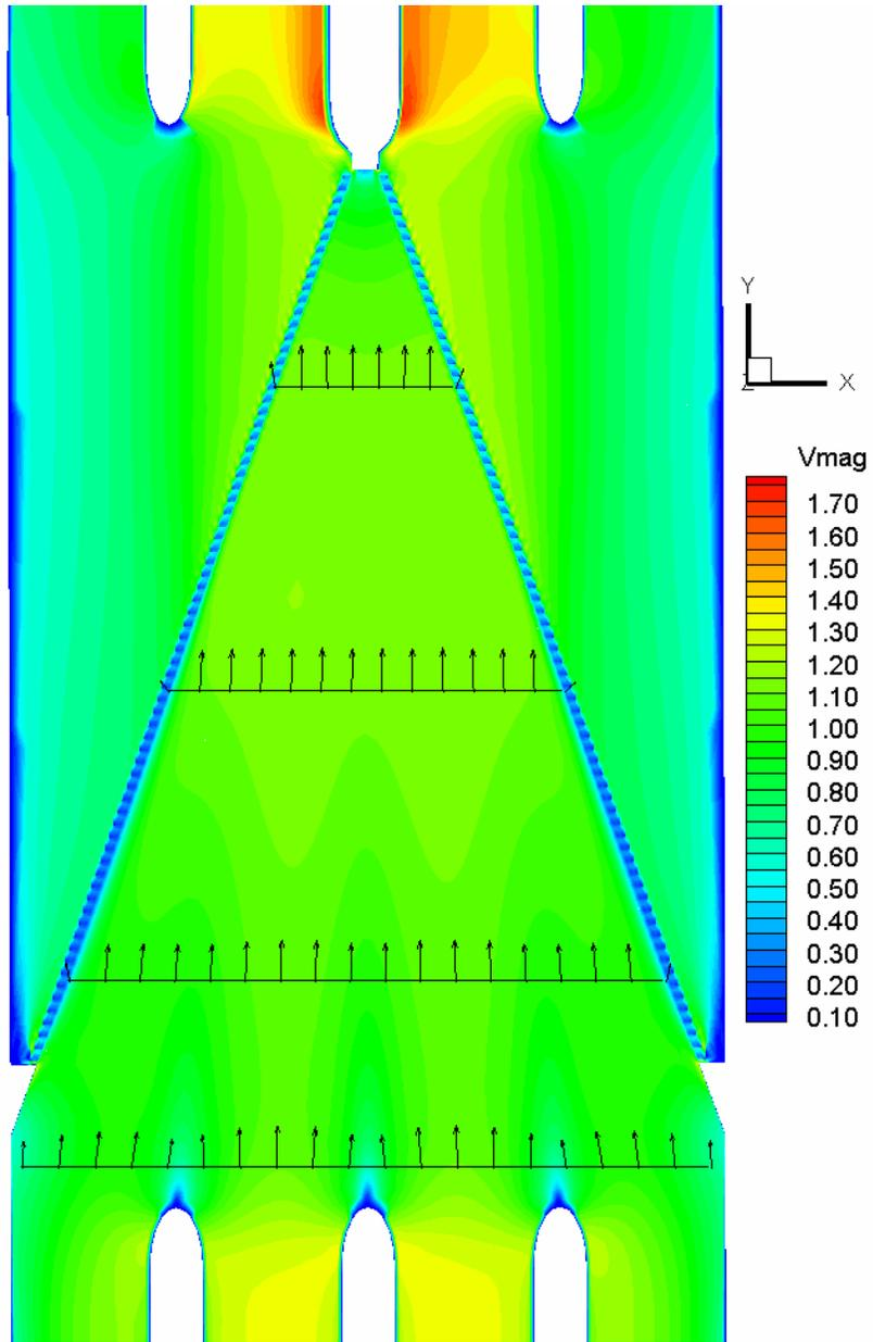
**Figure 9** – CFD predicted velocities at elevation 416.4 ft (msl) and 5,000 cfs.
