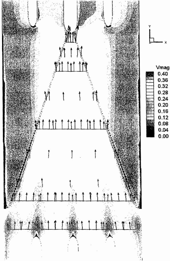
Figure C-5: Verification Run01 zoom view (Q=1290 cfs, elev. 402.7 ft, Vmag in m/s)
