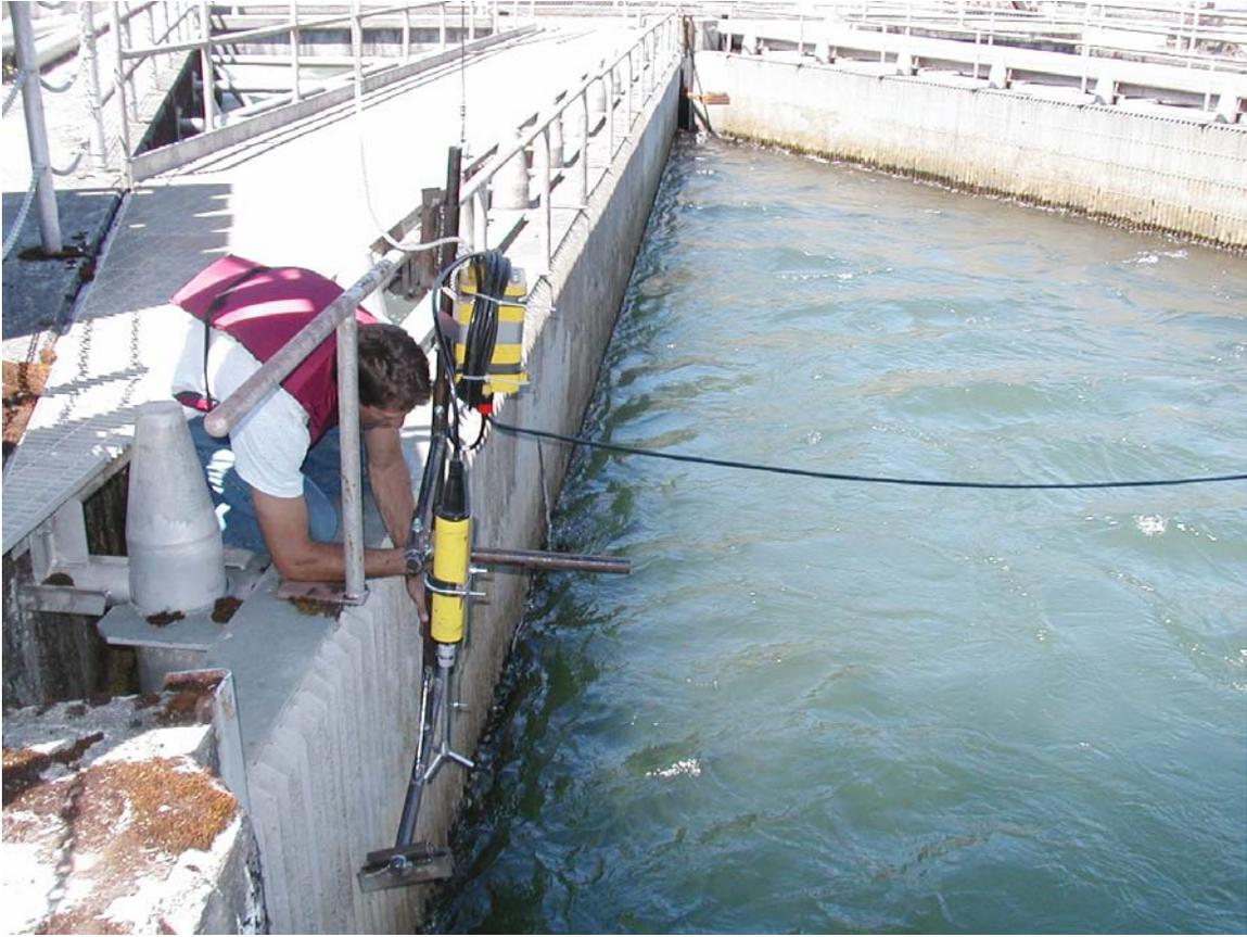
**Photo 2** - ADV probe mount shown on the left intake louver vanes.
