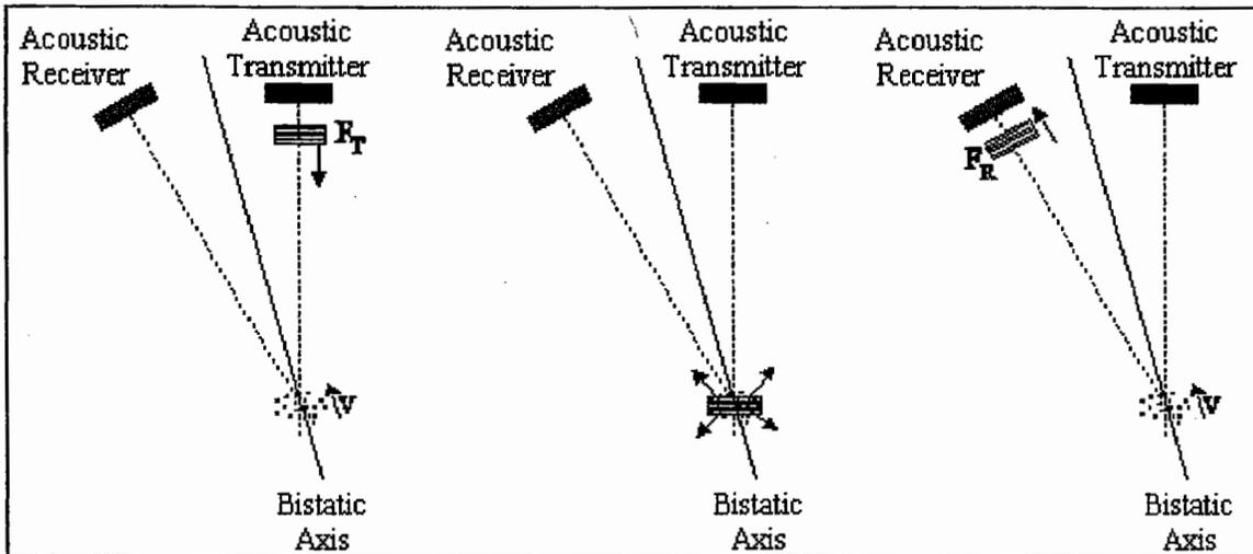
**Figure 3: Bistatic Acoustic Doppler Current Meter Operation**
