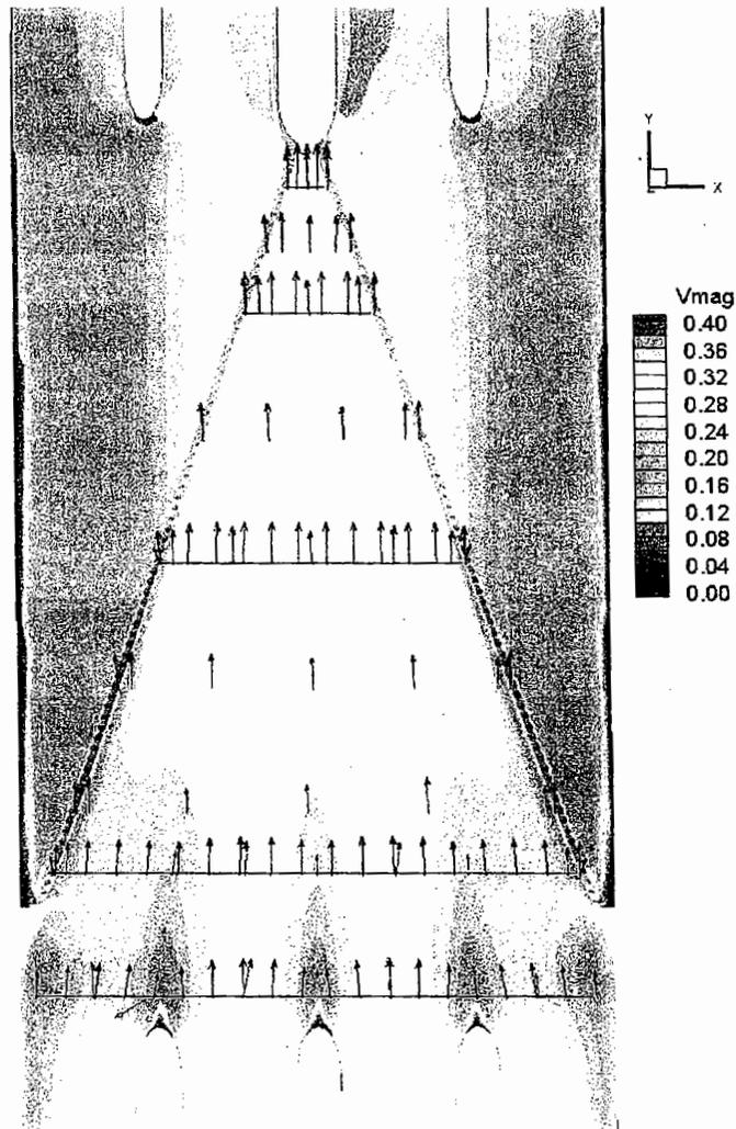
Figure C-8: Verification Run01 zoom view (Q=1290 cfs, elev. 416.4 ft, Vmag in m/s)
