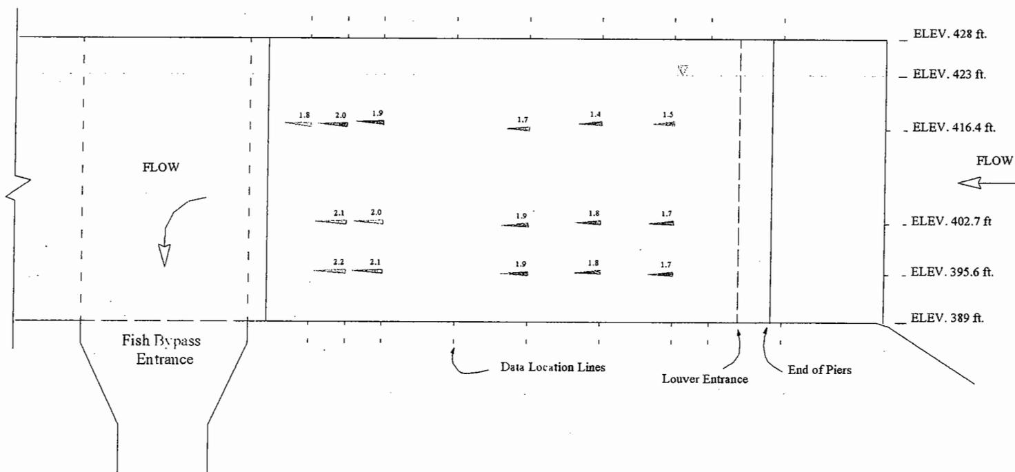
**Figure B-11: X-Z Vector Velocity (m/s) at Centerline (Q = 2580 cfs)**
