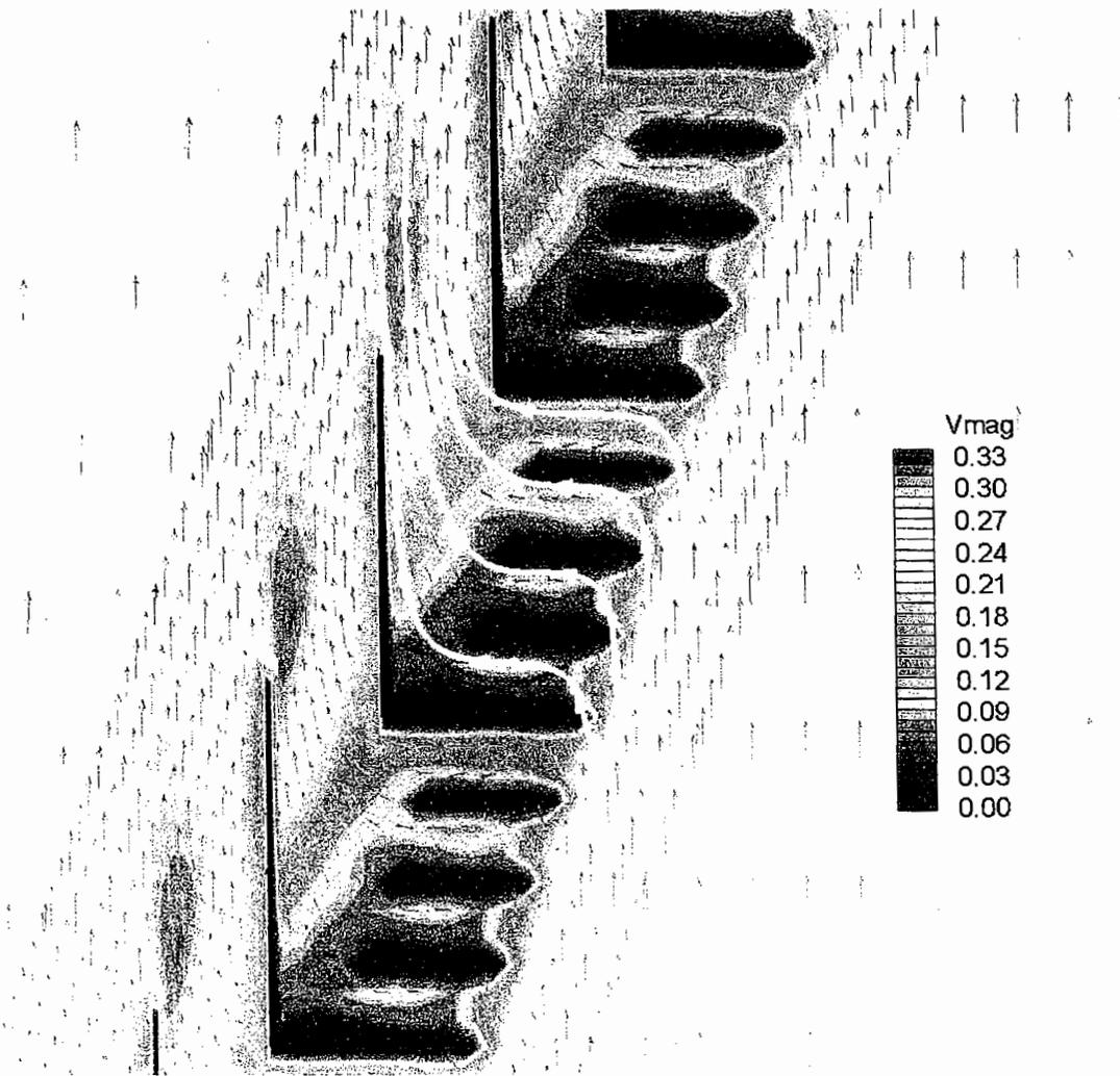
Figure C-21: Run05 louver zoom (Q=1290 cfs, elev. 416.4 ft, no-slip louvers, Vmag in m/s)
