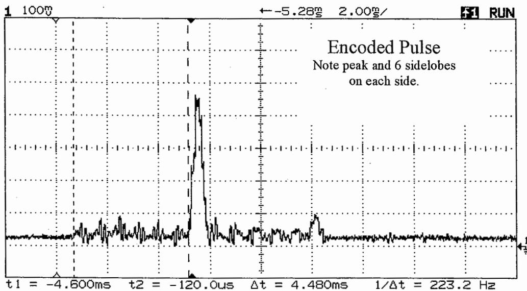
**Figure 11: Acoustic tag encoded pulse used in Mayfield Study. The peak amplitude of the pulse is the effective pulse width used for fish positioning. The surrounding peaks of lower amplitude are used by the 290 system to filter out background noise.**
