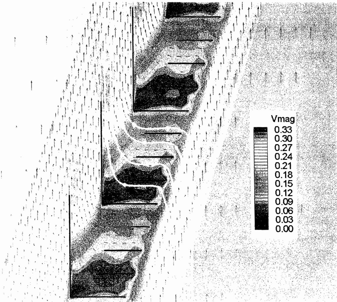
**Figure C-9: Verification Run01 louver zoom (Q=1290 cfs, elev.416.4 ft, free-slip louvers, Vmag in m/s)**
