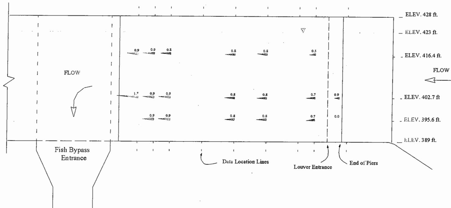
**Figure B-8: X-Z Vector Velocity (m/s) at Centerline (Q = 1290 cfs)**
