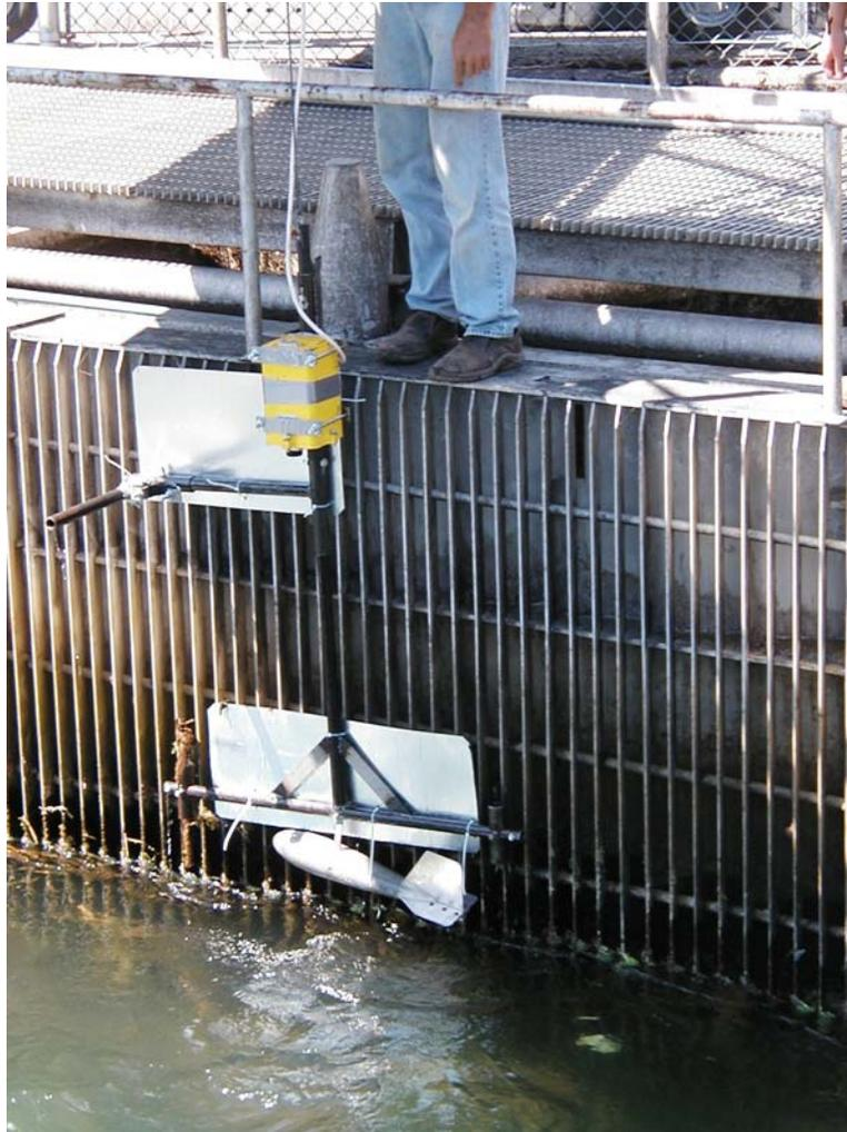
**Photo 4** - Instrument retrofitted with sheet metal panels and 100 lb lead weight.
