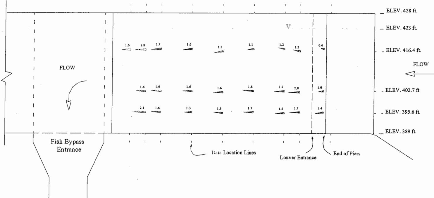
**Figure B-10: X-Z Vector Velocity (m/s) at East Louver (Q = 2580 cfs)**
