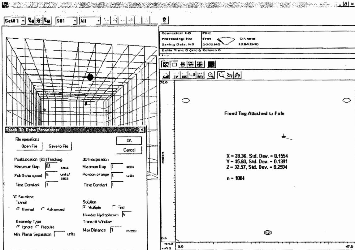
Figure 14: Plan view and 3-D view of stationary test results, including standard deviation of tag position error.
