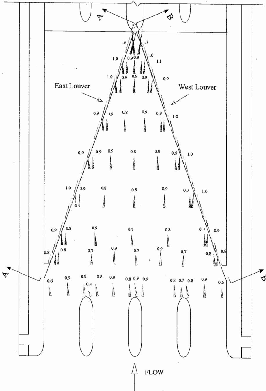
Figure B-2: X-Y Vector Velocity (m/s) at Elev. 402.3 ft (Q = 1290 cfs)
