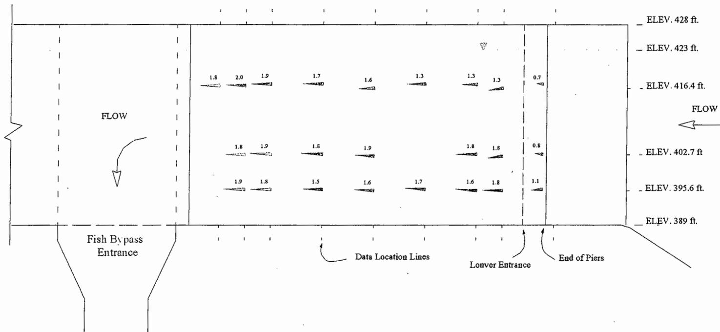
Figure B-12: X-Z Vector Velocity (m/s) at West Louver (Q = 2580 cfs)
