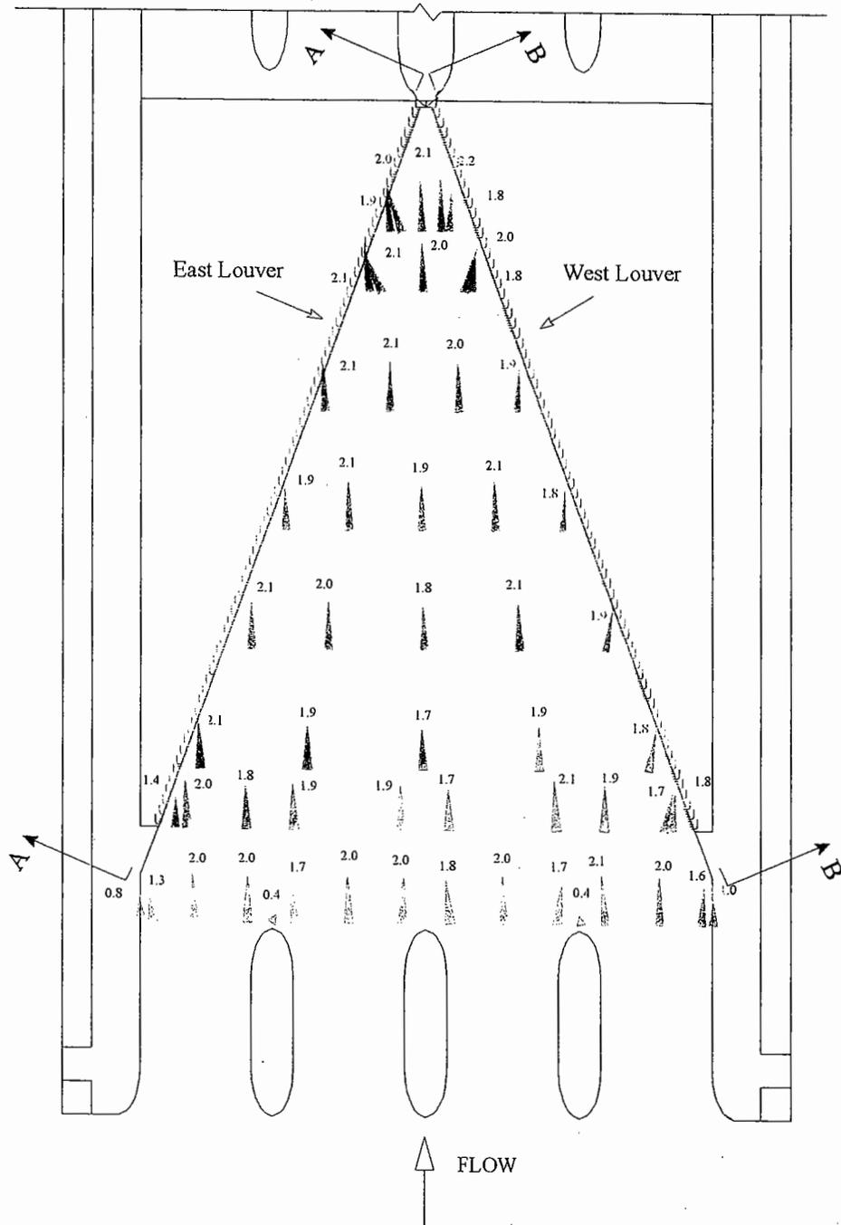
Figure B-5: X-Y Vector Velocity (m/s) at Elev. 402.3 ft (Q = 2580 cfs)
