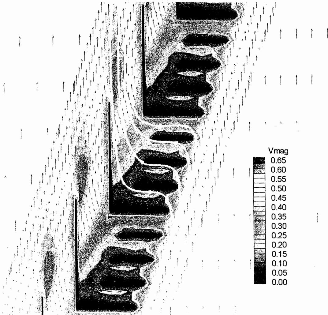
**Figure C-24: Run06 louver zoom (Q=2580 cfs, elev. 416.4 ft, no-slip louvers, Vmag in m/s)**
