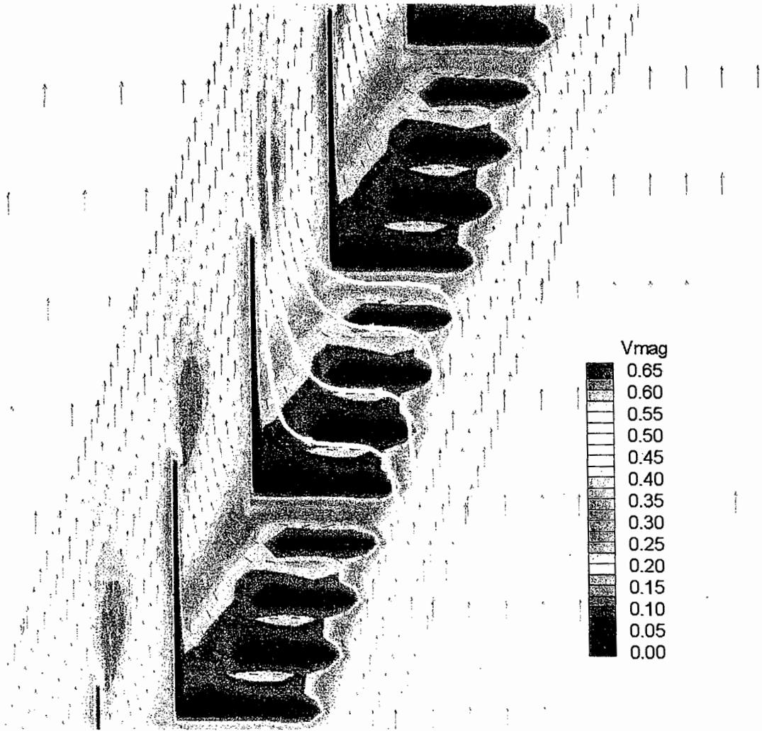
**Figure C-23: Run06 louver zoom (Q=2580 cfs, elev. 402.7 ft, no-slip louvers, Vmag in m/s)**
