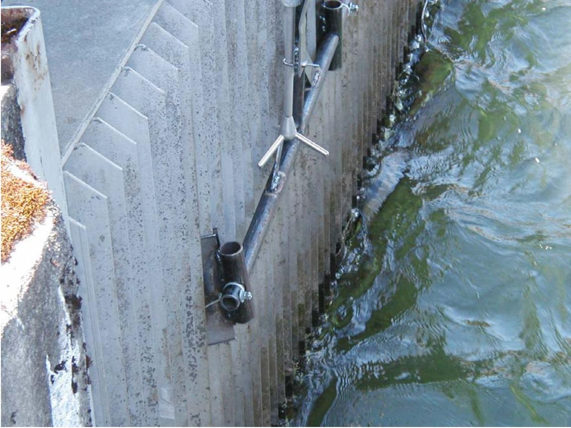
**Photo 3** - Zoomed view of ADV probe and louver vane indexing guides.
