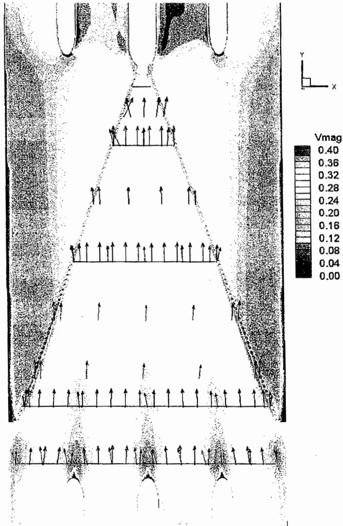
Figure C-2: Verification Run01 zoom view ( $Q=1290$  cfs, elev. 395.6 ft, Vmag in m/s)
