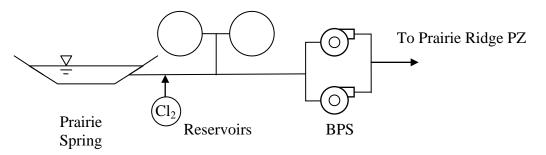
The reservoirs appeared to be in fair condition. *The vent screens were loose and need to be tightened.* Based on the schematic shown above it appears the reservoirs cannot be used for contact time in providing a CT of 6 to the spring.
