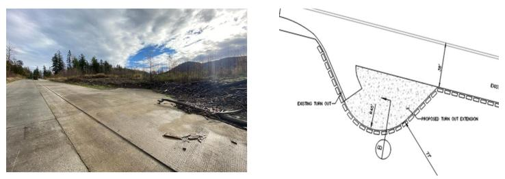
2) **Construction of a new anchor** at the bottom of the north launching lane to extend the reach of the courtesy dock to lower elevations (currently the dock is usable to about 731 feet, while the lane is usable to 719 feet; the new anchor will make the dock usable to about 726 feet).
