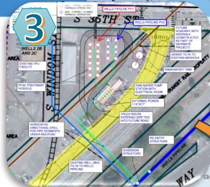
Wells Pipeline Treatment (Location TBD)
