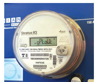
Radio Off Meter (displaying "opt-out on" its screen)
