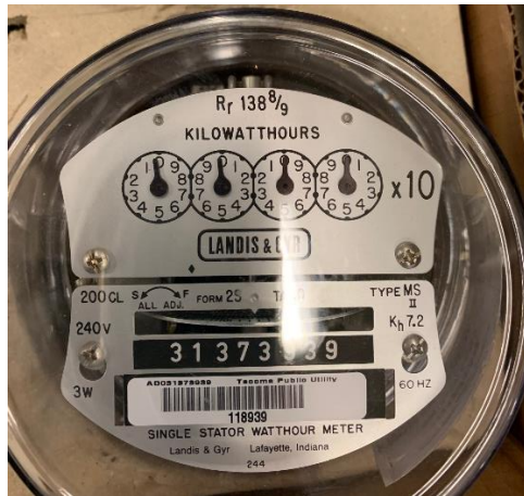
Legacy Electromechanical Meter
