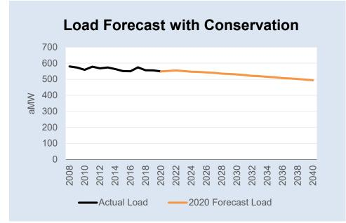
This chart shows a downward projection for our load. <u>Load</u> refers to energy consumption. Our system average load is projected to decline at a rate of approximately 0.44% per year, reflecting planned conservation measures.
