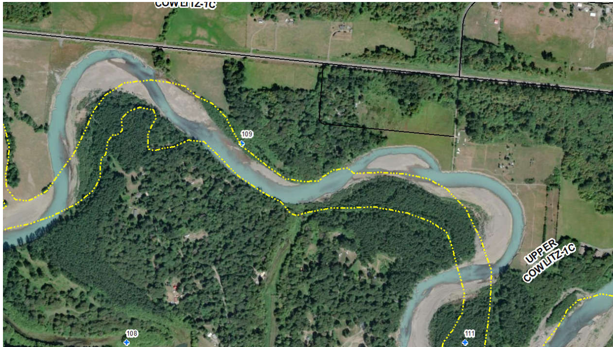
Figure 9. Current aerial photograph with 1994 unvegetated channel trace shown in yellow. Bank protection has been installed where the channel has migrated toward the highway.
