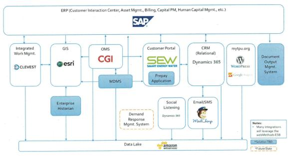
The diagram below is the tentative integration architecture for the first implementation of the Meter Data Management System ("MDMS") under this SOW.
