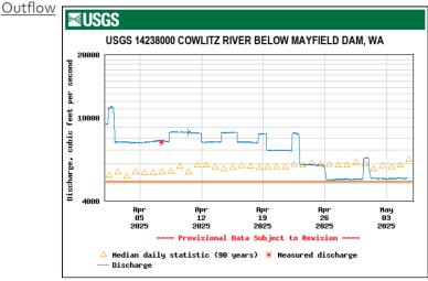
Current (5/5) discharge 5,160 cfs. 5,000 cfs min + weekly fish transport flow (if >8,000 cfs). Down ramping limits <6,000 cfs o in/hr day, 2 in/hr night. No exceedances.
